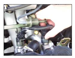
a. Remove the existing injector caps/plugs, by unclipping them. As shown in the photo on the left.
