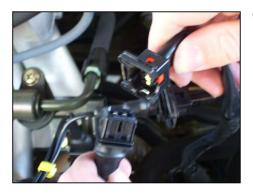
c. The photograph on the left shows the injector plug of the engine and the harness injector clip.
